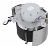
Cable reel inside the boom 臂内卷筒
